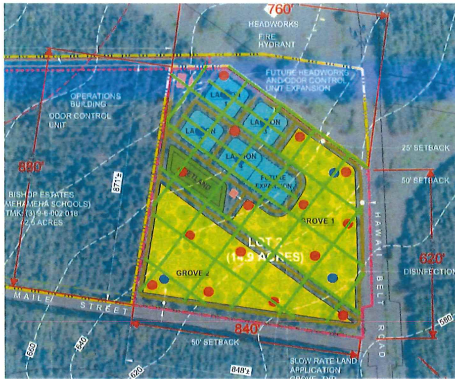
Insert 6 – Conceptual Locations of ERT and GPR Transects at the WWTP Site
